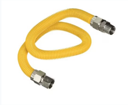
GF4 Yellow Gas Flex 48" Long 1/2" MIP x 3/4" MIP, 3/8" ID x 1/2" OD Yellow Gas Flex 48" Long 1/2" MIP x 3/4" MIP, 3/8" ID x 1/2" OD
